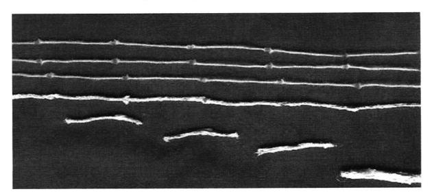
At the top, three pre-weakened strands, below them one that has been coated with a cement mix, three fibres broken off from such a strand. To the right a bundle of fibres, aligned & bonded together, as they can be randomly aligned in a mould.
