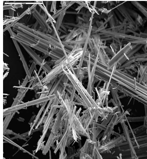
Chrysotile Asbestos fibres
