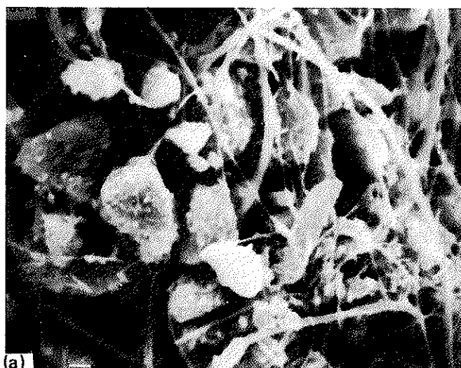
Figure 5 (a) Chrysotile fibres which are flexible are able to bend around cement particles ( \times 7K ). (b) By comparison, rigid crocidolite fibres ( \times 1K )
