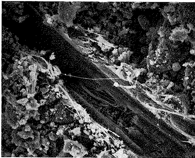
Figure 6 The outer sheath of chrysotile fibrils from a bundle remaining in a cement trough after separation and pull-out of the inner core ( \times 1K )
